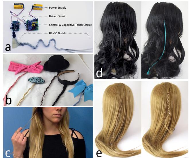
Figure 1. A) HäiriÖ prototype prior to miniaturization, B) exemplar HäiriÖ hair accessory form factors, C) HäiriÖ uses Swept Frequency Capacitive Sensing to detect natural hair interactions, D) HäiriÖ color changing properties using thermochromic pigments, and E) shape changing properties using Nitinol wire.
