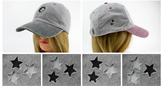
Figure 6. Baseball hat prototypes. Left: Hat prototype with AlterWear display on the front panel. Right: Hat prototype with AlterWear display on the side panel. Below: Close up of the side design. We added a simple animation when updating the display to give the appearance of sparkling or twinkling stars.
