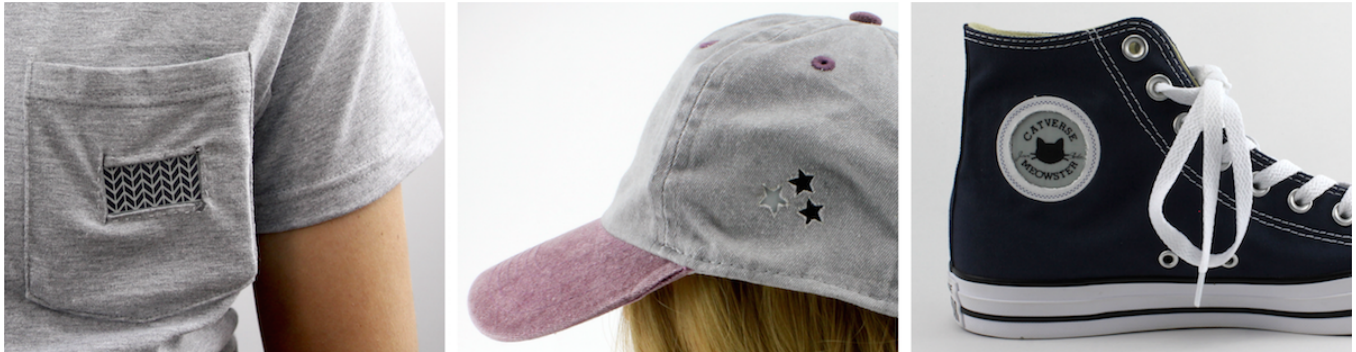
Figure 1. Three AlterWear prototypes. Note how well the technology is integrated into the garments. Left: Tee shirt pocket display (i.e. pattern). Middle: Segmented hat display (i.e. stars). Right: Discreet sneaker display (i.e. Catverse logo). AlterWear couples energy harvested from an NFC-enabled device with e-ink displays to afford dynamic interactions and expressions without the need for on-board power.
