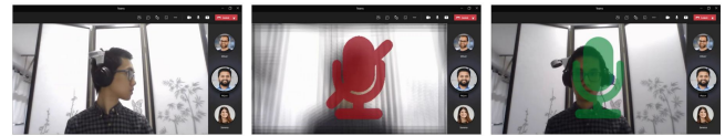
Figure 6: Context-aware privacy control. Left: A user disengages from a video call, reacting to a local conversation. Middle: The system infers the user’s intent to attend to something outside the known ecosystem of devices ( Environment Context ). As a result the video is blurred, the microphone is muted, and other users on the call are notified. Right: When the user returns to look at the screen, their video and microphone return to normal.
