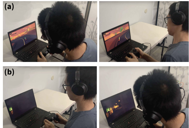
Figure 12: Leaning while wearing the headphone IMU impacts game play actions such as a) swerving the car to the side and b) peeking around the corner of a building.
