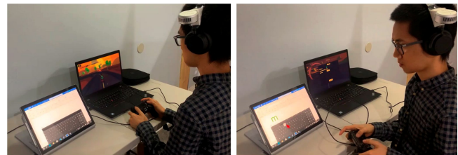
Figure 10: Augmented headphones can be used to manage other peripherals. In the picture to the right, the input from a game controller is redirected to the non-gaming device (the tablet).
