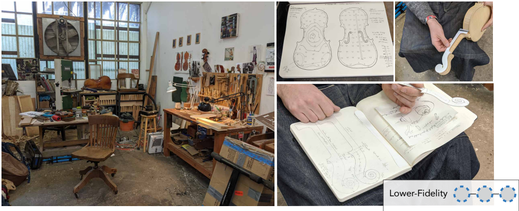
Fig. 6. The Violin Maker captures version histories in a variety of physical forms. From Left: The Violin Maker's workshop. Gradation diagrams used to record the depths of the top and back of a violin. Demonstrating a paper template for carving a neck and scroll on the partly-assembled instrument. The Violin Maker's notebook in which he records designs and modifications, showing versions of the neck template alongside the final template.
